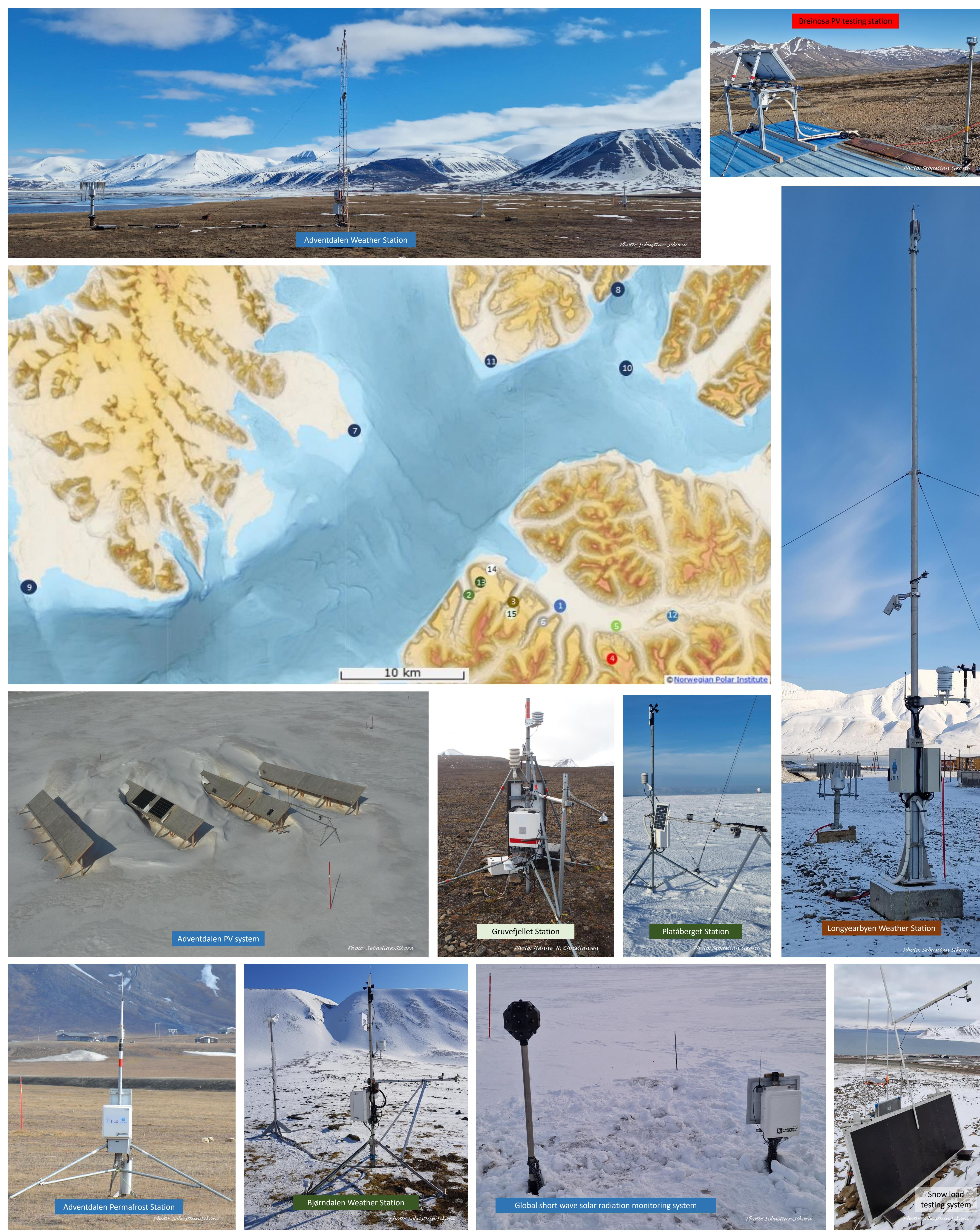
Most of the UNIS AWS stations are capable of transmitting data online, enabling real-time access to the collected information. In addition to standard observation systems, UNIS is pioneering the development of new systems to explore various aspects, including snow load on constructions, wind-related forces on photovoltaic panels, and the efficiency of photovoltaic modules in the Arctic.
