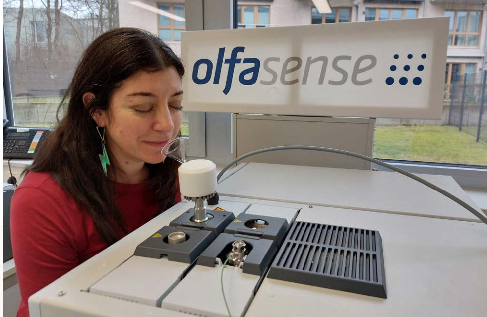
GC-MS analysis with olfactometric detection being conducted in an assessment study of smells in a museum. Photo courtesy of Cecilia Bembibre.
