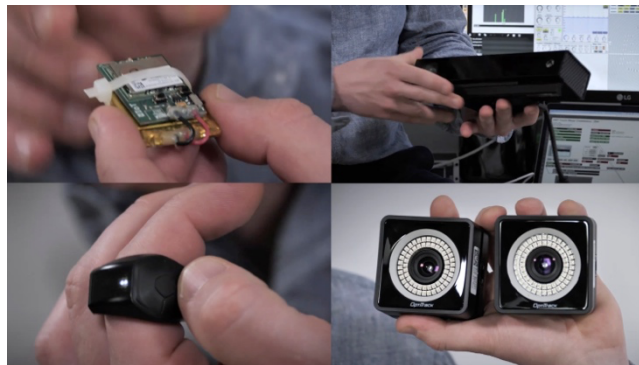
Fig. 1. Different hardware used to realize the instruments: Top left an XBEE sensor, bottom left a Genki Wave ring, top right a Kinect V2, bottom right two Optitrack cameras.
