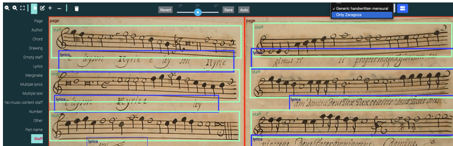
Fig. 2: Document analysis screen excerpt. In this example, only the staves and lyrics regions are segmented. The snapshot shows controls to rotate, manually or automatically, the image, and two possible classifiers to perform the operation automatically. The current catalog of region types shown at the left of the image can be easily modified.
