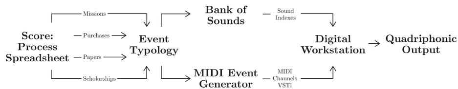
**Fig. 1.** The architecture of *soundscape4dei*: the Spreadsheet contains the data to be sonified, the Event Typology is described in the *Encoding* section, the MIDI events and Bank of Sounds are displayed in Table 1, and the digital workstation and quadriphonic output are detailed in the Instalation section.
