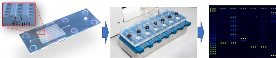
*Fig. 1: Multiplex system for allergen screening. Left, Picture of the microfluidic system; middle, image of automated microfluidic system; right, the fluorescent signals on the micropillars*
