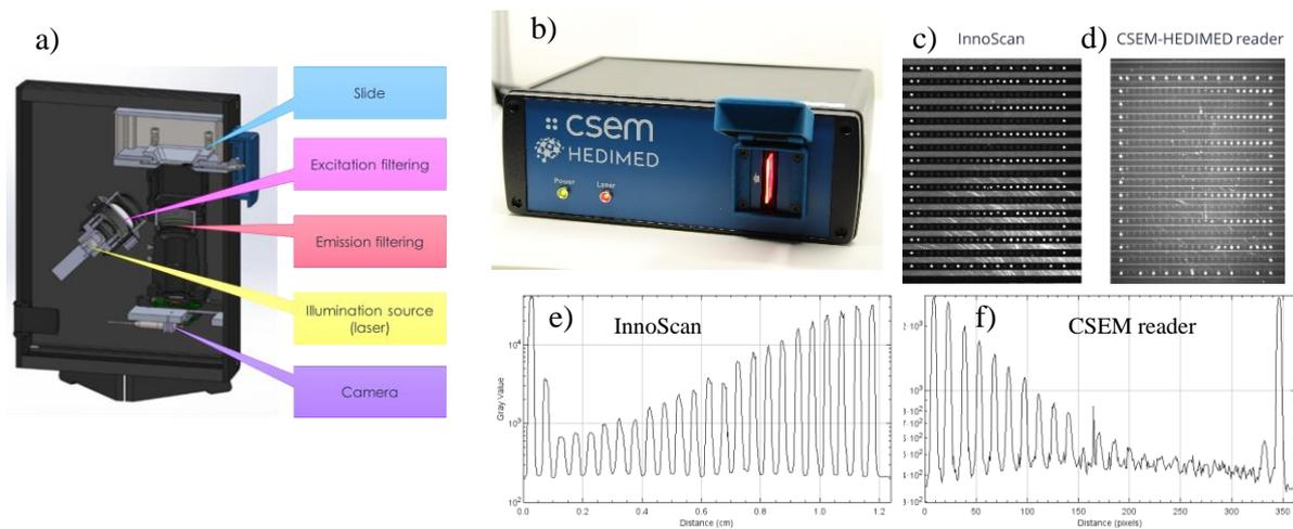
Fig. 2: a) Portable fluorescence reader structure; b) photo of the portable reader; c,d) comparison of the data acquired by InnoScan and the portable reader; (e,f) correspondent line profile in log-scale
