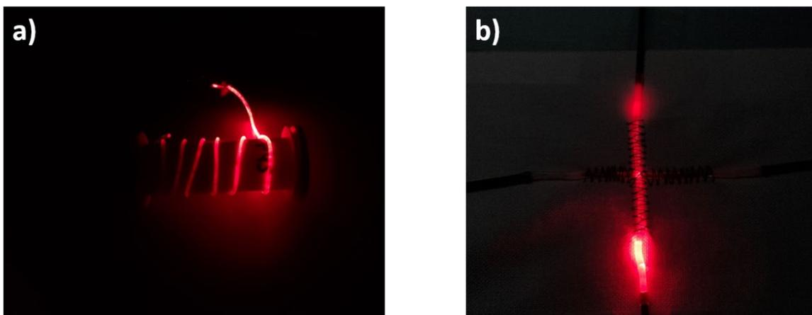
**Figure 1.** Digital images of soft PDMS POFs produced via MWS. a) POF showing successful transmission of light at the wavelength of 660 nm. b) Developed textile integrated soft POF based wearable optical sensor demonstrating transmission of red light with wavelength of 660 nm.
