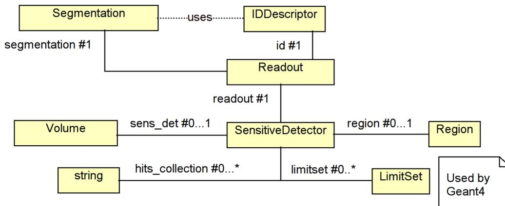
Figure 7: The structure of DD4hep sensitive detectors.
