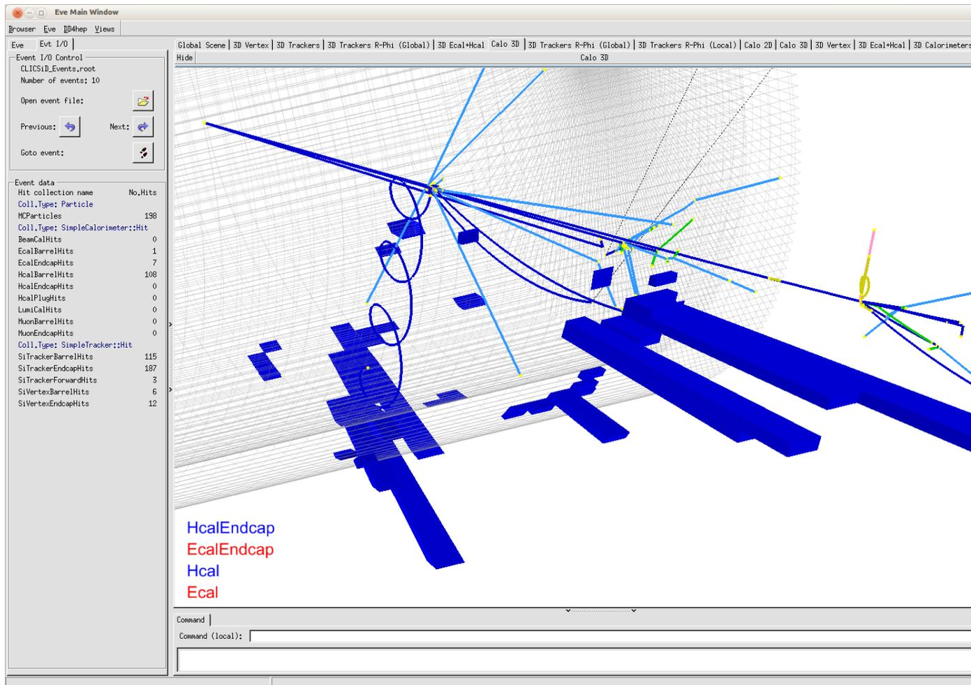
Figure 7: HCAL calorimeter deposits together with Monte-Carlo tracks.
