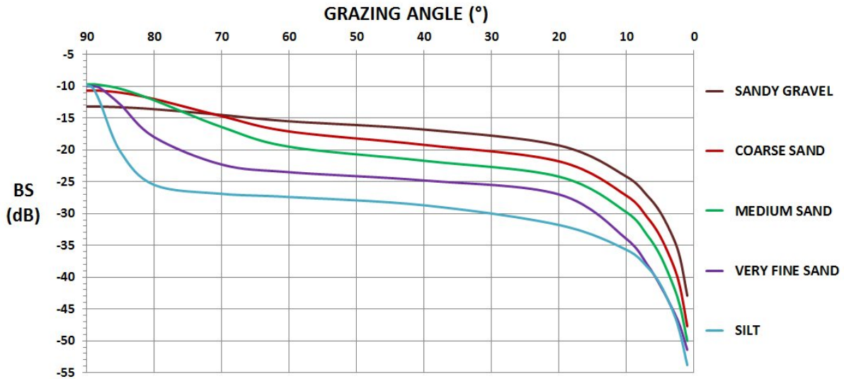
Figure 3-6 Backscatter Strength (BS) versus grazing angle for different classes of sediment at 100 kHz. Data from: University of Washington Applied Physics Laboratory, high-frequency ocean environmental acoustic models, APL-UW TR 9407-AEAS 9501, October 1994.
