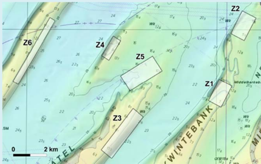
Figure 5-5 MBES (Kongsberg EM3002D on R/V Belgica) backscatter survey areas during a five year study, varying from fine to coarse sand.
