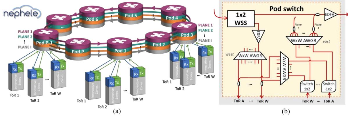
Figure 1: (a) NEPHELE architecture; (b) Block diagram of NEPHELE pod switch.
