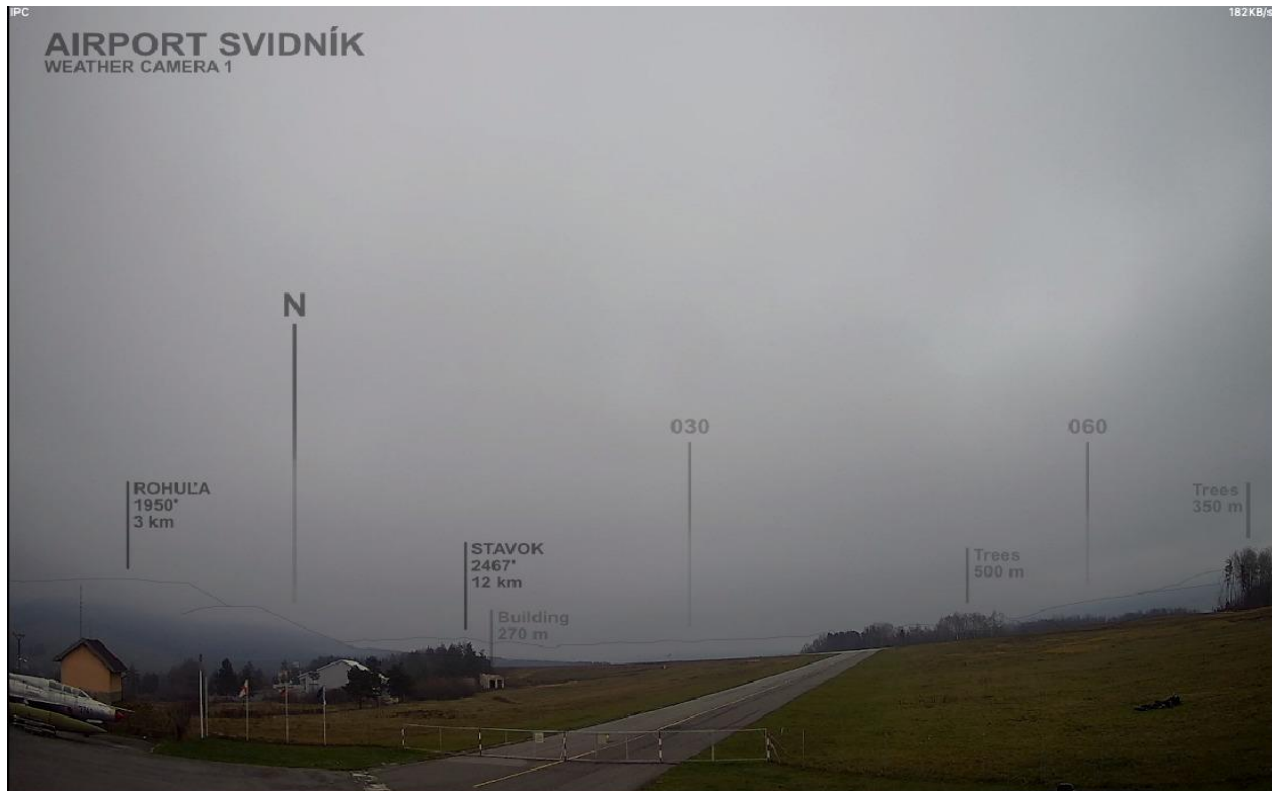
Figure 6. Visibility and cloud determination using a webcam. Source: own source
