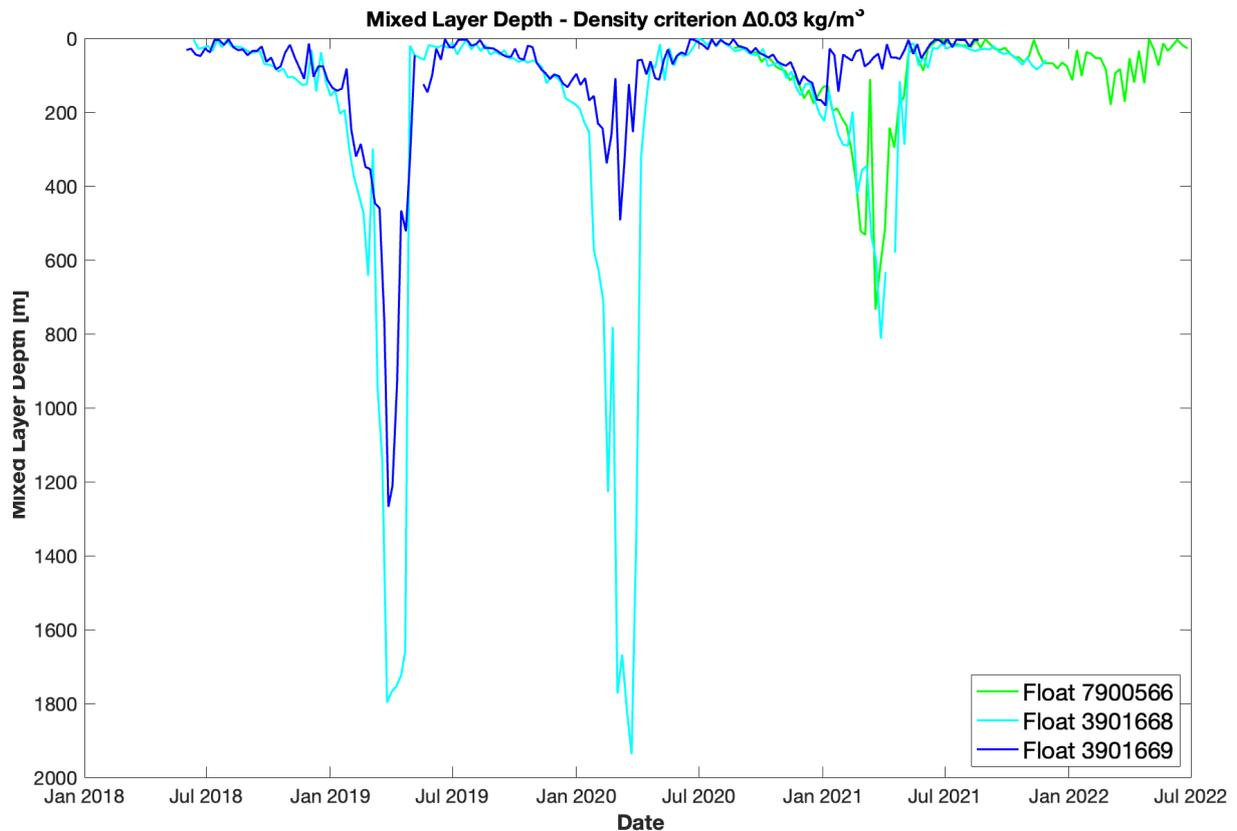
**Fig. 7:** Mixed layer depth in the Labrador Sea region based on the observation from three floats of our pilot study (WMO 3901668, WMO 3901669, WMO 7900566). An MLD threshold criterion in potential density of  $\Delta\sigma = 0.03 \text{ kg m}^{-3}$  from the value at 10 m was chosen.
