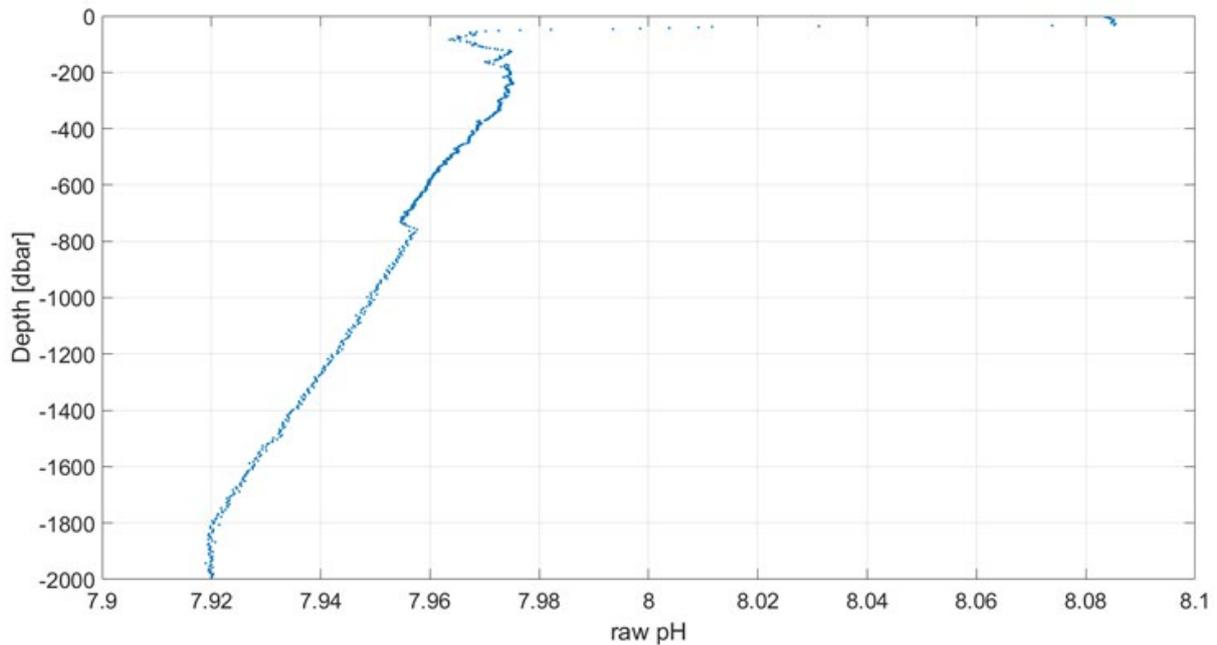
**Fig. 3:** Example of the step-like jump in the pH profile that occurred when the CTD pump was switched on during at 700 dbar profiling (Apex float).
