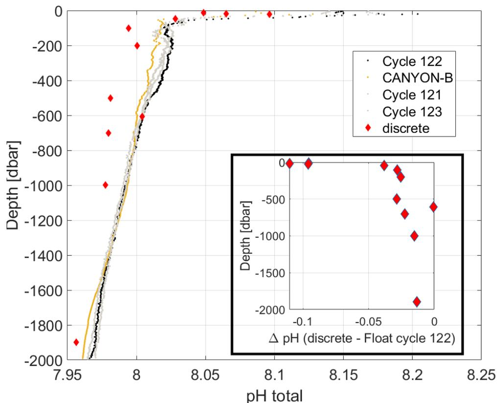
**Fig. 10:** WMO 3901669 pH profiles 121, 122 and 123 (corrected to the CANYON-B/CONTENT reference profile) and the discrete pH reference profile corrected to in-situ temperature and pressure (left panel) and absolute pH differences (discrete minus float) after matching in density space.
