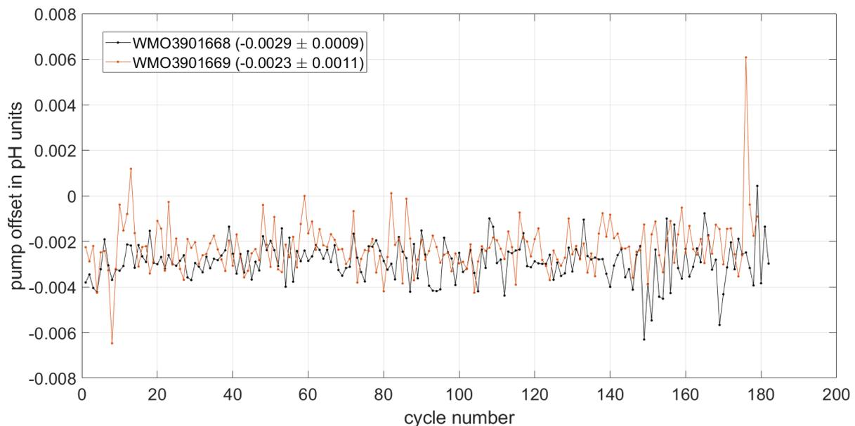
**Fig. 4:** Time series of the estimated pump offset during the lifetime of floats WMO 3901668 and WMO 3901669.
