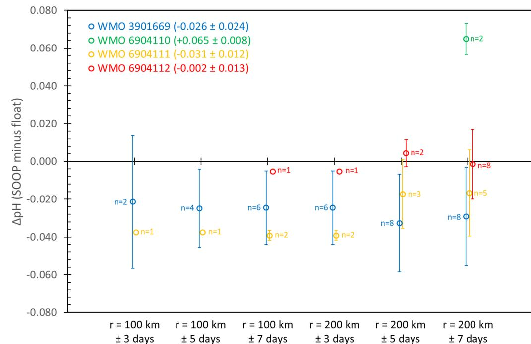
**Fig. 12:** Offset between SOOP pH and fully corrected float pH at crossovers. The 6 sets of criteria applied in the crossover search are shown at the bottom of figure. For each set of criteria the average pH offset ( $\pm 1\sigma$ ) is shown together with number of crossovers found. No further selection criteria were applied. The legend provides for each float the average offset ( $\pm$  mean  $1\sigma$ ) across all sets of selection criteria.
