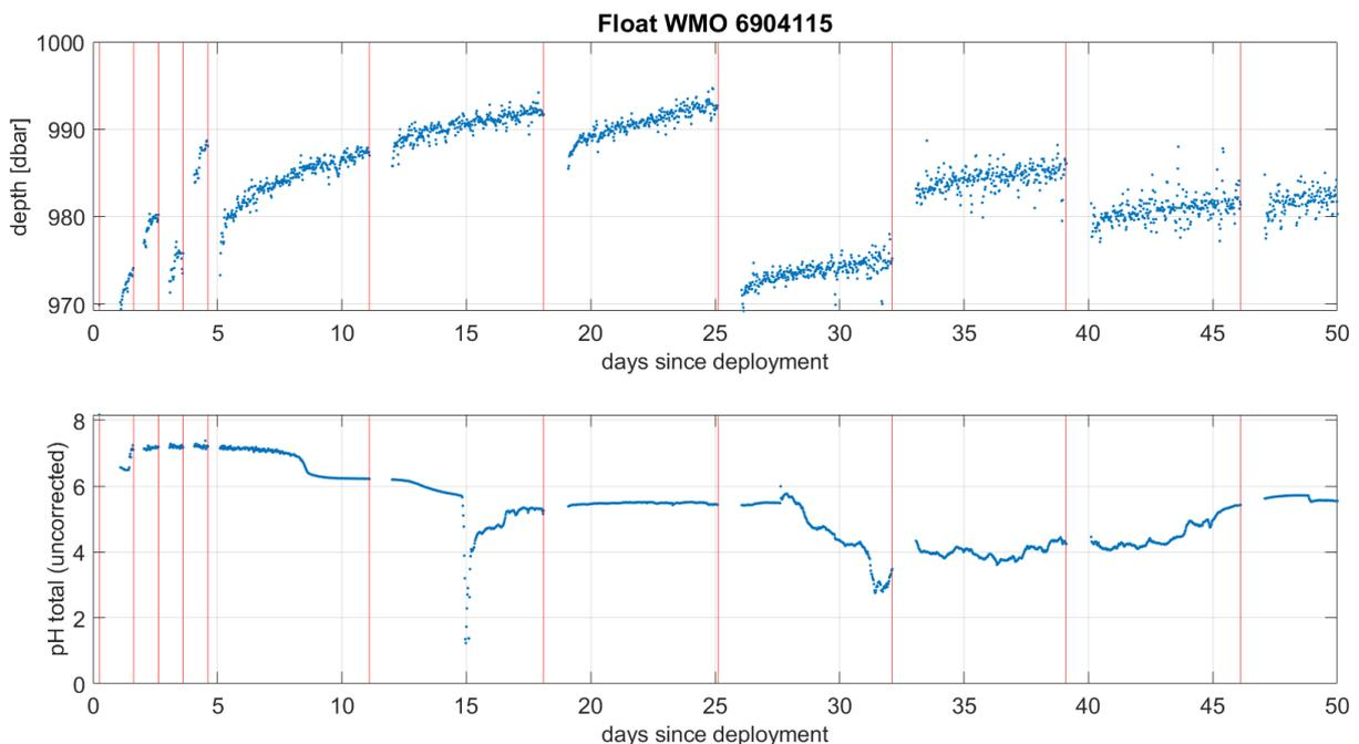
**Fig. 9:** Time series of pH measured by float WMO 6904115 at drift depth (1000 dbar) since deployment. Only data between park start (PST) and end time (PET) shown. Red lines indicate time of profiling.
