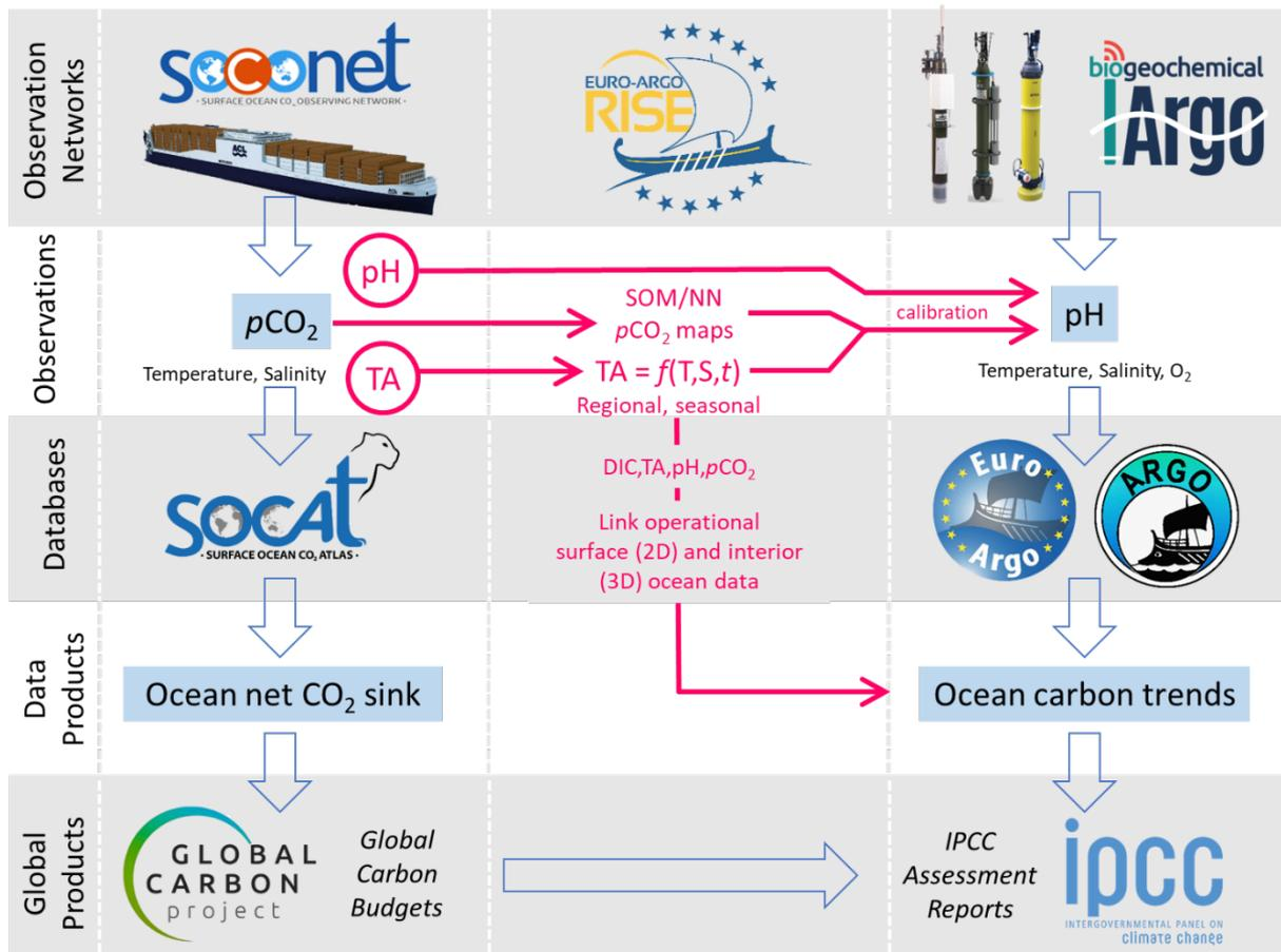
**Fig. 1:** Concept for synergistic coupling of SOCONET and BGC-Argo observatories in the context of marine carbon observations.
