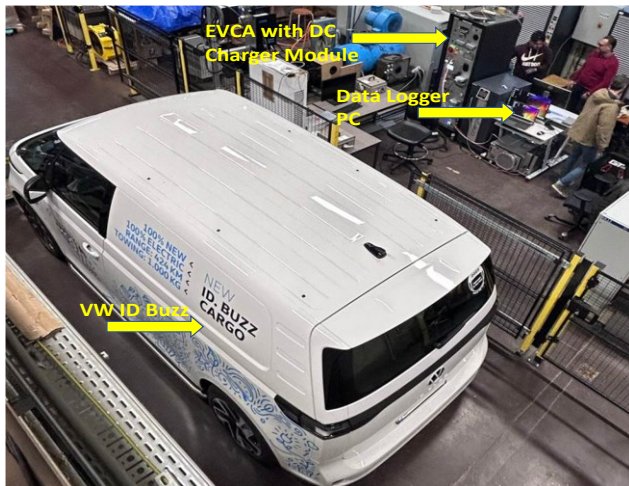
Fig. 11: The laboratory test system setup for charging and V2G for VW ID Buzz.
