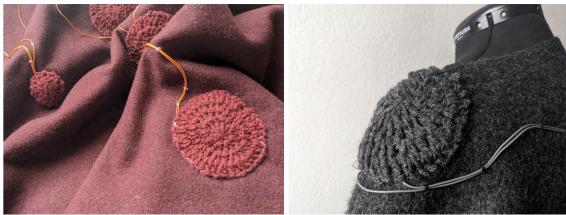
Figure 3. Fabric speakers and electronic components have been sewed inside crochet patches
