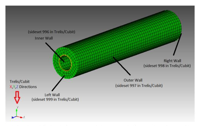
With the sidesets defined in the figure, we provide here an example of a minimal set of command line options:
