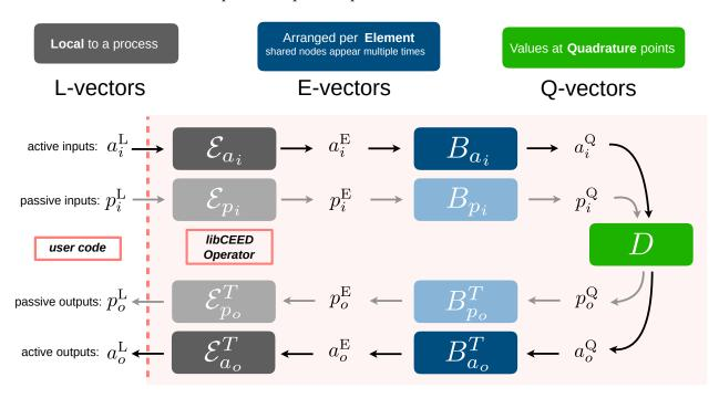
Fig. 3.2: Flow of data through vector types inside libCEED Operators, through backend implementations of  $\mathcal{E}$ ,  $\mathbf{B}$ , and  $\mathbf{D}$
