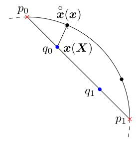
Fig. 4.2: Sketch of coordinates mapping between a 1D linear element and a circle. In the case of a linear element the two nodes,  $p_0$  and  $p_1$ , marked by red crosses, coincide with the endpoints of the element. Two quadrature points,  $q_0$  and  $q_1$ , marked by blue dots, with physical coordinates denoted by x(X), are mapped to their corresponding radial projections on the circle, which have coordinates  $\mathring{x}(x)$ .
