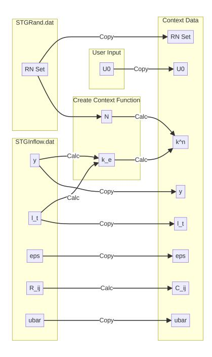
This is done once at runtime. The spatially-varying terms are then evaluated at each quadrature point on-the-fly, either by interpolation (for  $l_t$ ,  $\varepsilon$ ,  $C_{ij}$ , and  $\overline{u}$ ) or by calculation (for  $q^n$ ).
