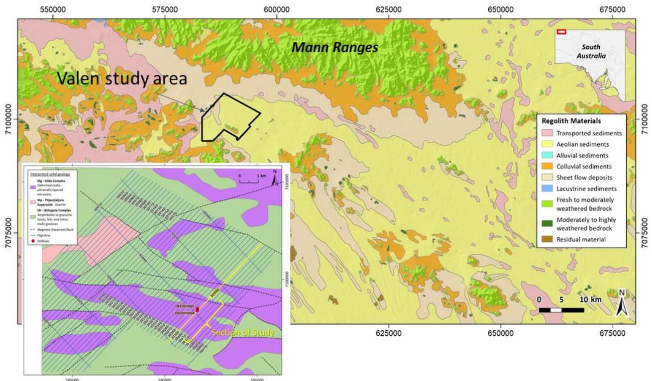
**Figure 1: Regolith geology of Valen Prospect area with inset map showing flight lines form VTEM survey and sub-set of the line investigated here. The drillholes marked by the red circles are coincident with the Valen late-time anomaly observed in the AEM data sets.**
