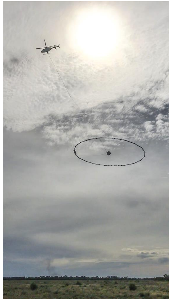
Figure 12: The transmitter in flight, with a 3 component BIPTTEM sensor in the centre
