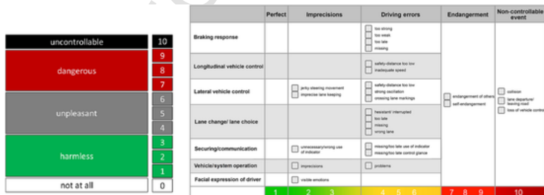
Fig. 1. Subjective criticality rating scale (left) and rating sheet for the TOC-rating showing the detailed error categories (right).
