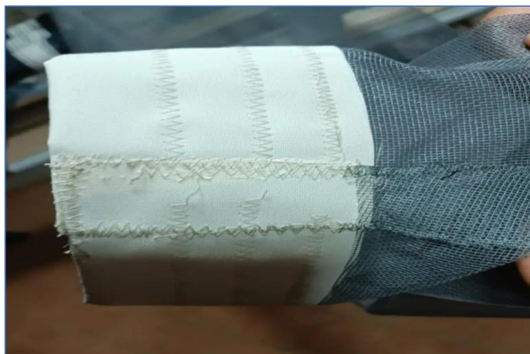
Figure 9. Detail on how the tearproof nylon fabric and the net were sewed together.
