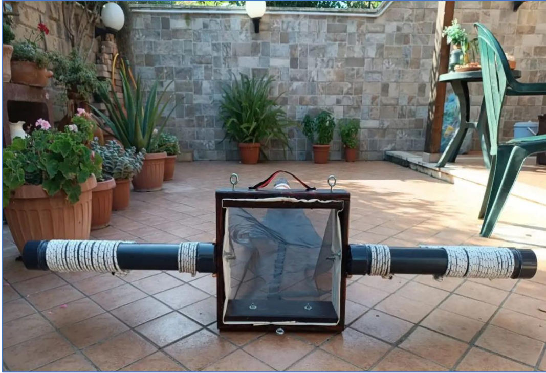
Figure 11. The front of the LADI device with the three eyelets visible, on which the carabiners of the towing ropes will be attached.
