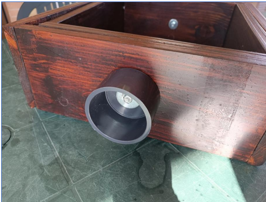
Figure 5. The mouth rectangles (inner and outer), with the central end cap bolted on the outer rectangle. This end cap hosts the central tube of the three tubes that constitute each of the wings of the LADI.
