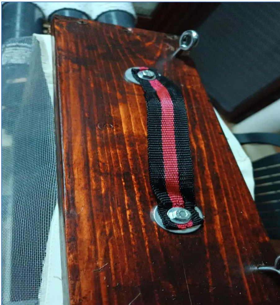
Figure 4. The strap fixed on the upper outer rectangle side, to ease the handling of the device.
