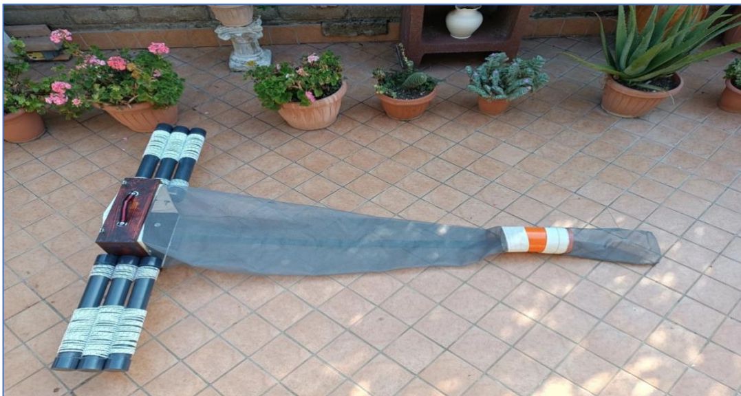
Figure 10. The complete LADI device. Note the left wing has a backward inclination towards the lower back-end of the structure of about 7 degrees. This allows the mouth to stay afloat.
