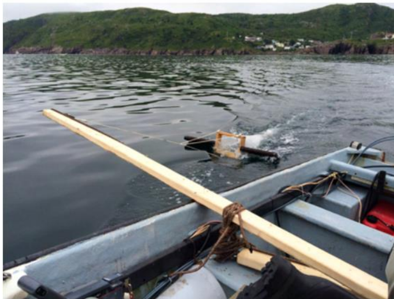
Figure 12. A trawling arm to trawl the LADI laterally and avoid the wake. Image from “LADI and the Trawl” by Coco Coyle with Melissa Novaceski, Emily Wells and Max Liboiron, as published by the Civic Laboratory for Environmental Action Research, August 2016.
