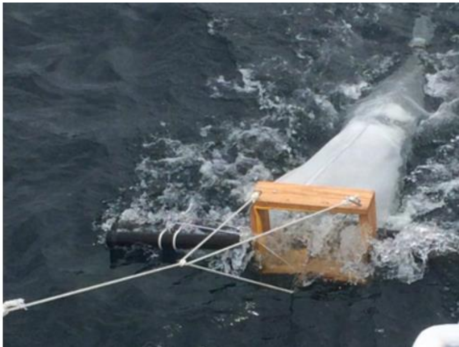
Figure 14. How the LADI trawl is attached, from the original document (Coyle et al., 2016, the Civic Laboratory for Environmental Action Research).
