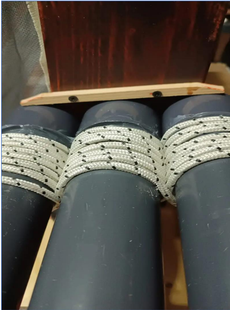
Figure 6. Fixing the wings with ropes.
