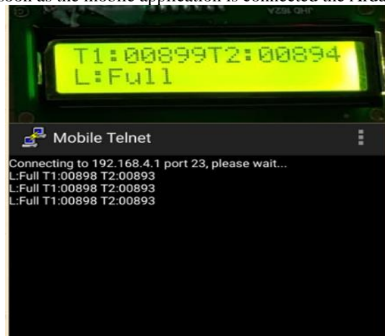
Fig 3: Displayed output of Engine Oil Impurities and level Monitoring System
