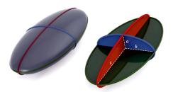
Figure 1.1: A three-dimensional *tri-axial* ellipsoid (*i.e.* a < b < c). The diagram on the right shows all three semi-principle axes: the semi-minor axis, a; the semi-intermediate axis, b and the semi-major axis, c. [3]
