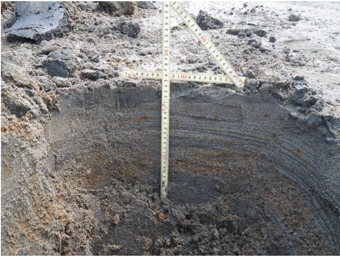
Figure S2. The tsunami deposit at Loc. 1 (See Figure 1C and Figure S1 for location and lithofacies). The sand layer exhibits a distinct normal grading structure and parallel lamination.
