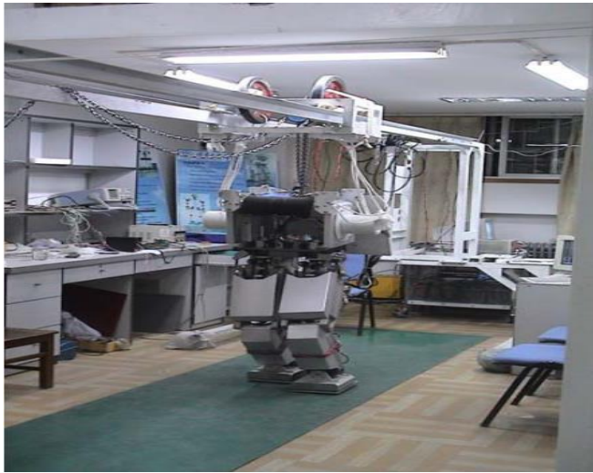
Figure 1: THBIP-I humanoid robot [1,8]
