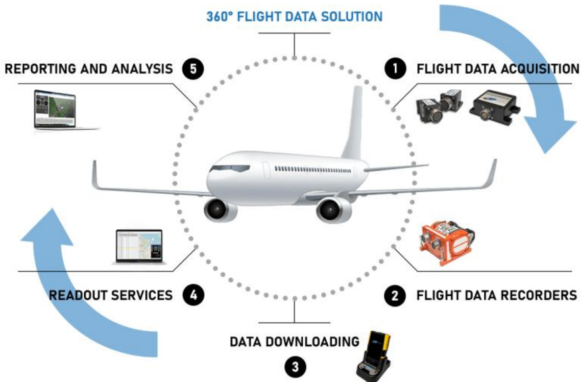
Figure 2: The life cycle of flight data in FDM.
