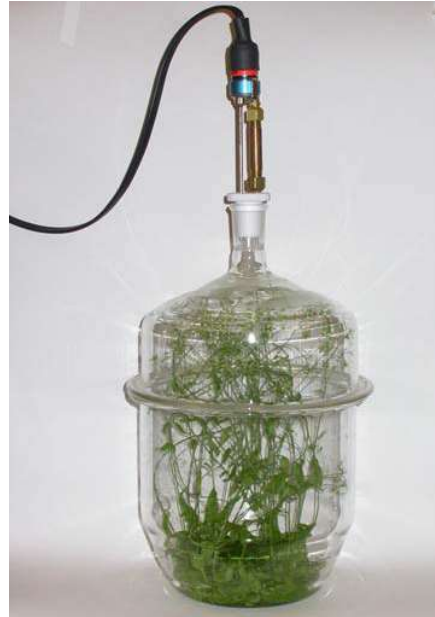
Figure 2. The dynamic headspace collection set.
