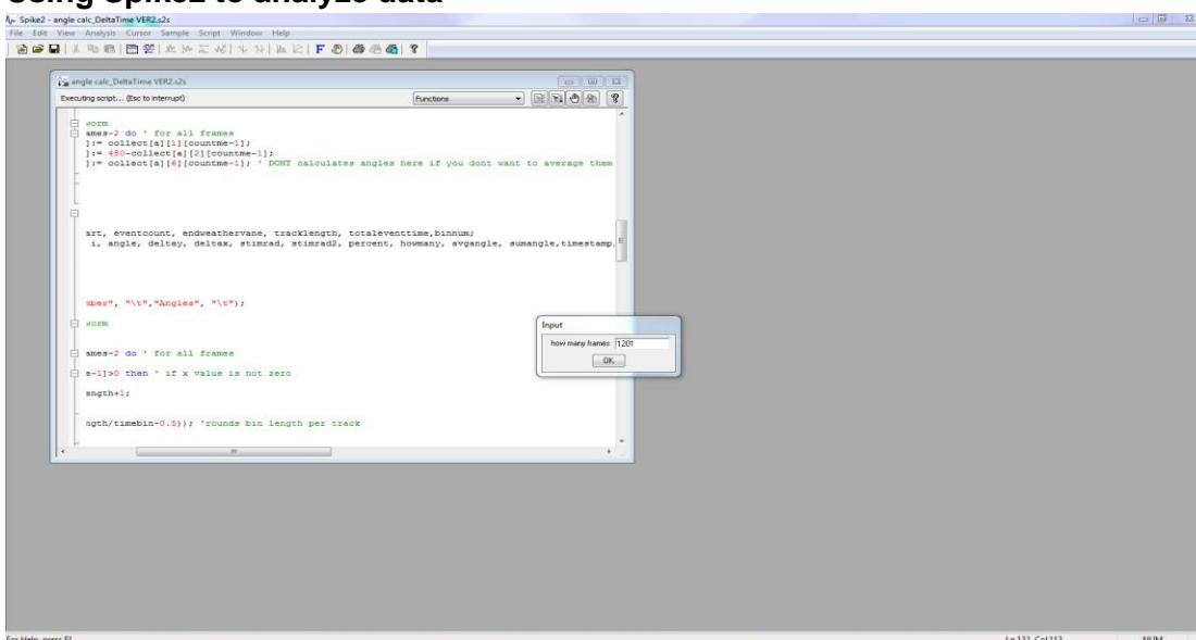
Run the script using the tab delimited files. Frame number should be reported as n+1 frames (e.g. if there are 1200 frames in a video, 1201 should be reported to the script.) When asked if you want to “plot in sequence” select “n” and hit OK.
