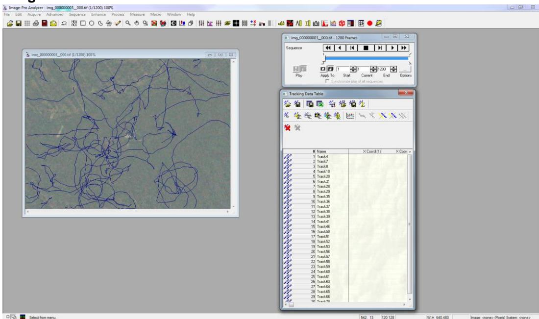
Tracking data (X, and Y coordinates) should be exported to Microsoft Excel by hitting the green “excel button”, and then saved as a tab delimited file from within Microsoft Excel. It is important to note the frame number of video being analyzed. Data from this tracking set is included in this submission.
