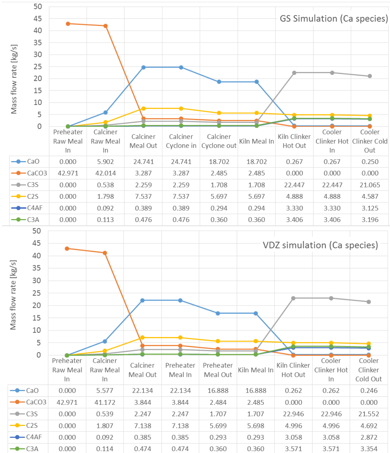
Figure 3.3 Mass flow rate of the calcium-based species along the cement kiln sections in the GS and VDZ simulations. The mass flow rates are related to the main stream (dust recirculation is not included).
