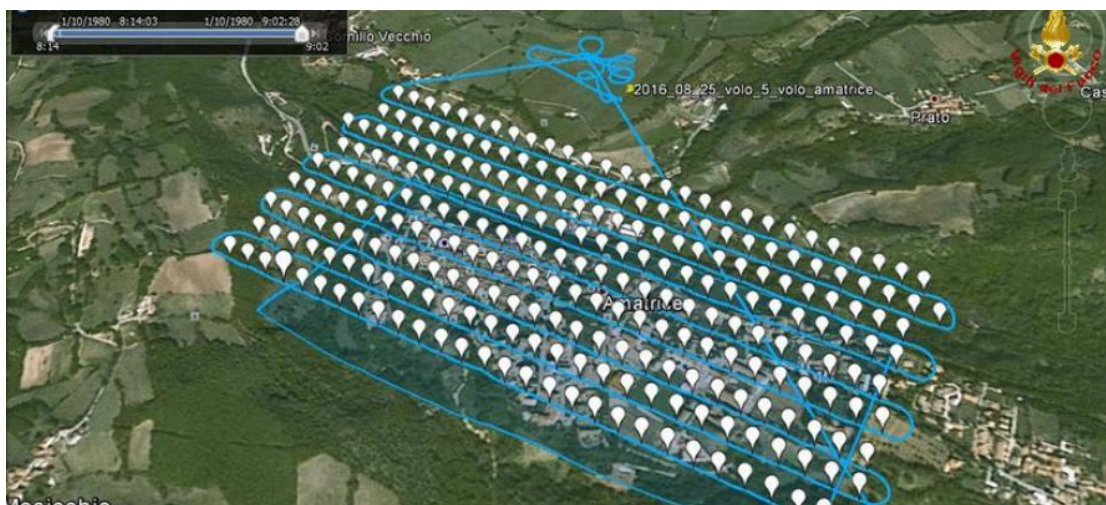
Fig. 7. Flight plan of a drone operated on the town of Amatrice in the aftermath of the August 24, 2016 earthquake.
