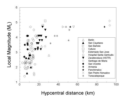
Figure 4. Magnitude-distance distribution of swarm data, indicating accelerograph station from which each recording was obtained. Information on the accelerograph stations is reported in Bommer *et al.* (1997).
