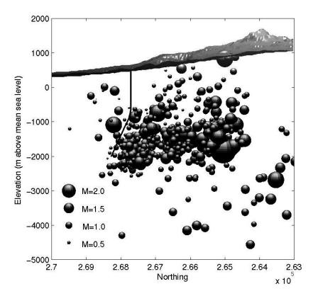
Figure 8. Cross-section of the seismicity at the Berlín field as recorded by the micro-seismic network during the entire period of fracture stimulation, including the intervals between periods of injection. Northing coordinates are given in meters. The black line shows the TR8A injection well. The largest event (265000N, elevation -2000) is the earthquake of 16 September 2003 (see Section 4.2)
