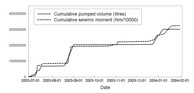
Figure 10. Comparison of cumulative volume of pumped liquid (litres) and induced seismicity (in terms of cumulative seismic moment). The seismicity occurred in the area bounded by coordinates 267000-268800 N and 551000-554000 E.
