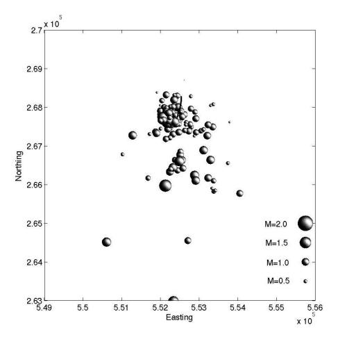
Figure 9. Epicentral map of seismic events during the fracture stimulation period (coordinates are expressed in meters). The black line is the projection of the TR8A injection well.
