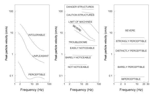
Figure 2: *Left*: Recommended levels of human sensitivity to vibration due to blasting from the USACE (1972); *Middle*: Reference levels for vibration perception and response from traffic, adapted from Barneich (1985); *Right*: thresholds for vibrations due to pile-driving from Athanasopoulos and Pelekis (2000)
