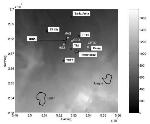
Figure 7. Map of the Berlín geothmermal field and surrounding area showing the location of the seismographs (black symbols) and accelerographs (white symbols). The gray scale indicates the ground elevation (in metres) with respect to sea level; the Eastings and Northings are given in metres.
