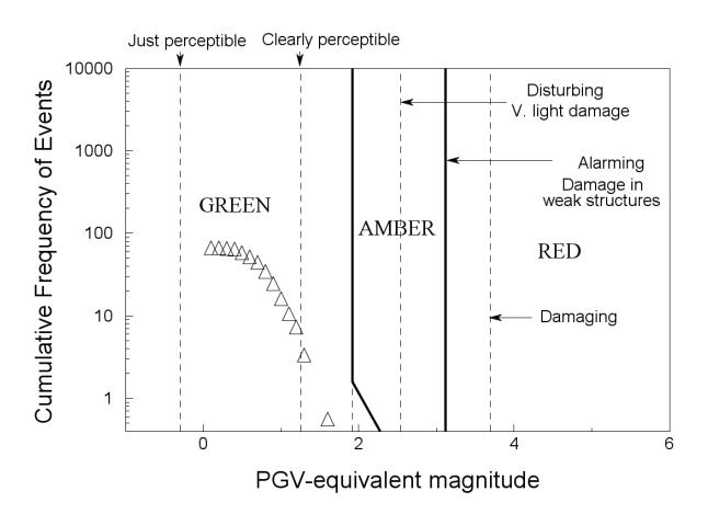
Figure 6. "Traffic light" boundaries superimposed on recurrence defined in terms of magnitudes adjusted to produce the same epicentral PGV if their focal depth was exactly 2 km. The triangles represent the cumulative recurrence data from the three episodes of pumping (totalling 54 days of pumping) normalized to a period of 30 days
