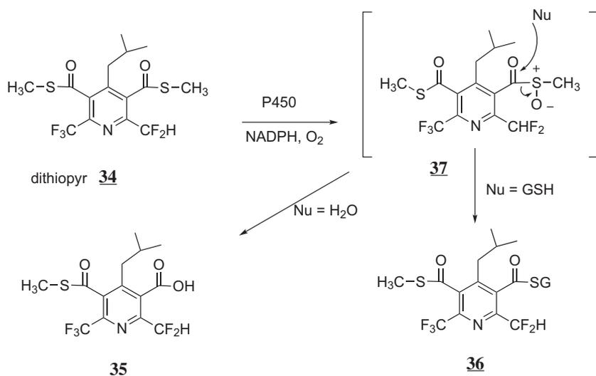
**Fig. 16.** Formation of a reactive intermediate during metabolic transformation of the thioester functions of dithiopyr into carboxylic acid functions.
