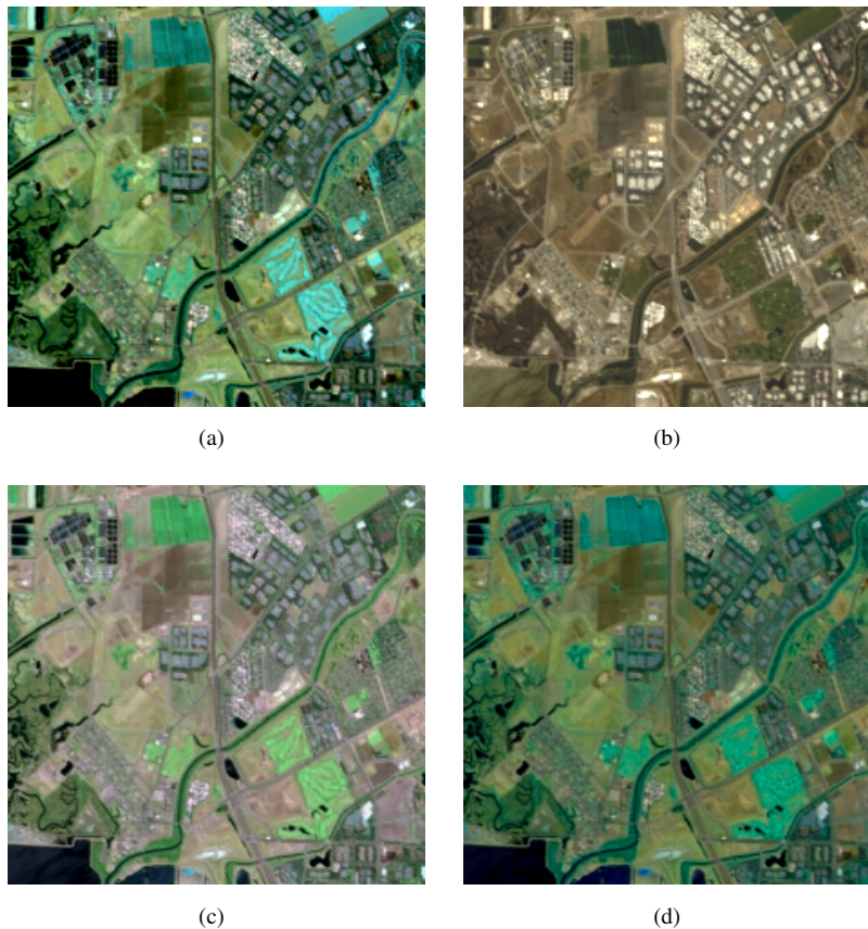
Fig. 4: Visual comparison of performances of various image fusion approaches over a block of the Moffett field hyperspectral image cube (Moffett02) shown in Fig. 2d. Results of fusion using (a) proposed method after tristimulus display of fused images shown in Figs. 2(a-c), (b) three band selection approach, (c) piecewise linear function approach, and (d) color matching function approach. Gamma is set to 1.5 for all color displays.
