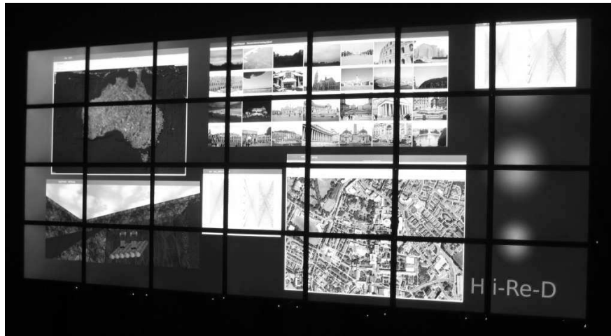
FIGURE 1: A 54 million pixel Powerwall made of 28 x 20-inch TFT monitors. The wall measures 3.02m by 1.32m.
