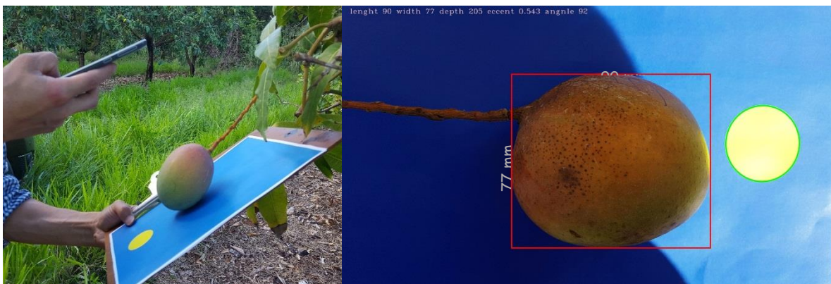
Figure 4. In-field imaging (left) and the result of fruit sizing mobile app (right)
