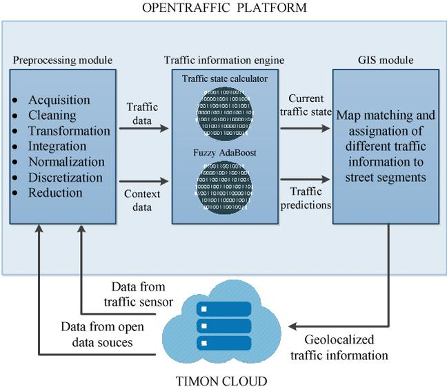
**Figure 2 - OT platform process for the traffic predictions and current traffic state data distribution**
