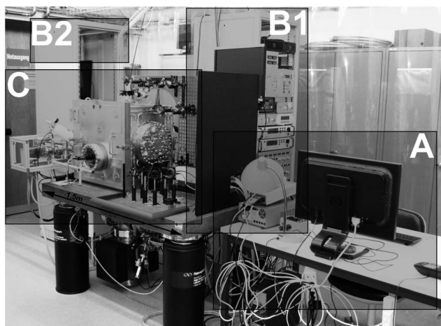
Fig. 1 Overview of the instrument setup in the laboratory. (A) represents the remote control station; (B1/B2) the electronic equipment, e.g. measurement computer, power supplies, etc.; (C) the instrument setup itself. Detailed information about part (C) can be found in Fig. 2.
