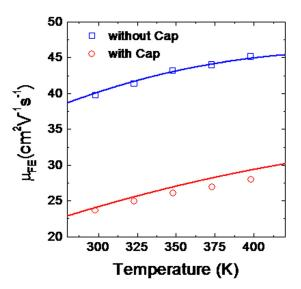
FIG. 2. Temperature dependence of the field effect mobility ( $\mu_{\text{FE}}$ ) for the devices processed with or without a capping layer. The continue lines are the theoretical fit obtained with two different values of the trapped charge density.
