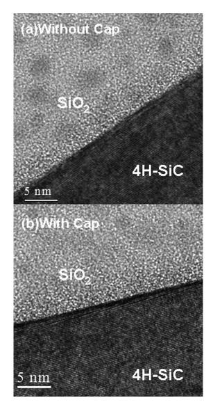
FIG. 4. High resolution transmission electron microscopy images of the gate region (SiO<sub>2</sub>/4H-SiC interface) in the lateral MOSFET processed under the two different conditions. The images were taken along the [1-100] zone axis, which is perpendicular to the [0001] direction of 4H-SiC.
