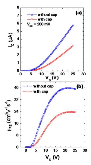
FIG. 1. (a) Drain current (I<sub>D</sub>) as a function of gate bias (V<sub>G</sub>) for lateral 4H-SiC MOSFETs processed either with or without using a capping layer during post-implantation high-temperature annealing: (b) Field effect mobility ( $\mu_{FE}$ ) as a function of V<sub>G</sub> determined by the MOSFETs transfer characteristics for the two annealing conditions.
