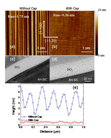
FIG. 5. AFM morphologies of the 4H-SiC surfaces treated without (a) and with (b) the capping layer, and corresponding cross sectional TEM micrographs of the SiO<sub>2</sub>/4H-SiC interfaces ((c) and (d)). (e) AFM single scanned line taken on the surfaces of the two samples.
