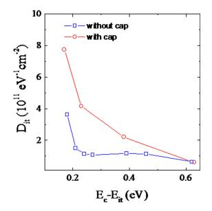
FIG. 3. Interface state density  $\left(D_{it}\right)$  measured on the 4H-SiC MOS fabricated on the same wafers
