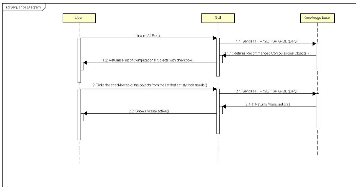
**Diagram 1:** Sequence diagram showing software component interactions for natural language input method.
