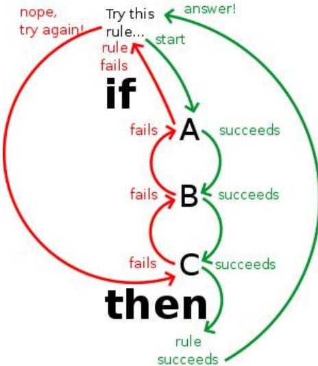
**Figure 1:** Backtracking example flow.
