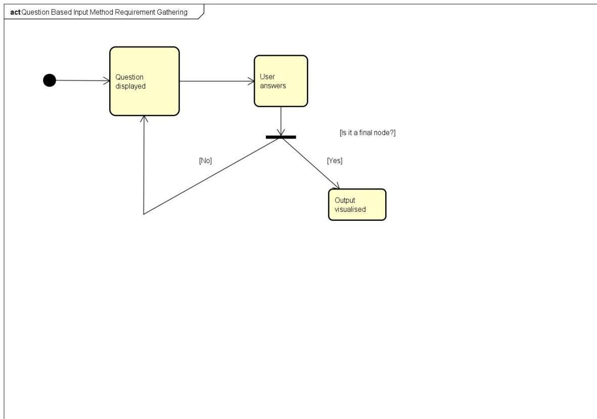
**Diagram 5:** Activity Diagram for the question-based input method.
