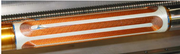
Figure 5. The ALPHA superconducting octupole being wound. The wire is about 1 mm thick and when fully powered holds a current of about 1000 A.
