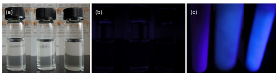
Figure 2 Photographs of the solutions of starch (left), cellulose (middle) and BSA (right) taken at room temperature (a, b) and 77 K (c) under room lighting (a) and 365-nm UV illumination (b, c).
