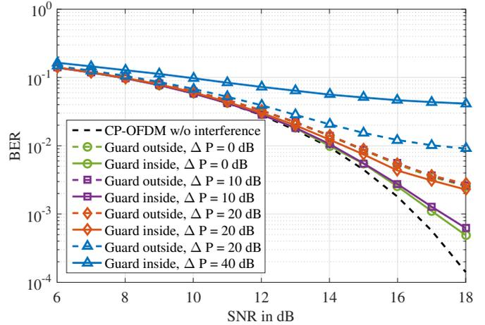
Fig. 9. Uncoded BER performance of F-OFDM on an AWGN channel with 2 guard SCs and 16QAM modulation.
