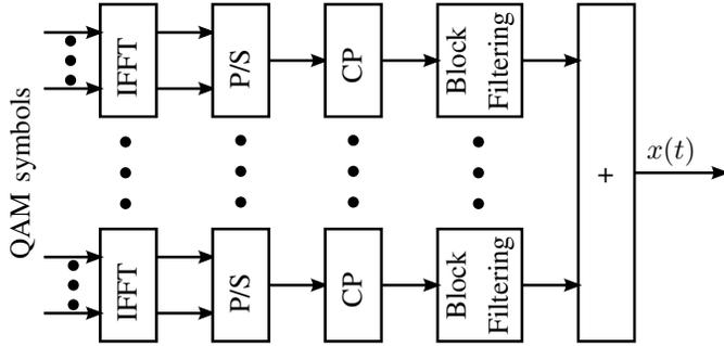
Fig. 1. F-OFDM block diagram.
