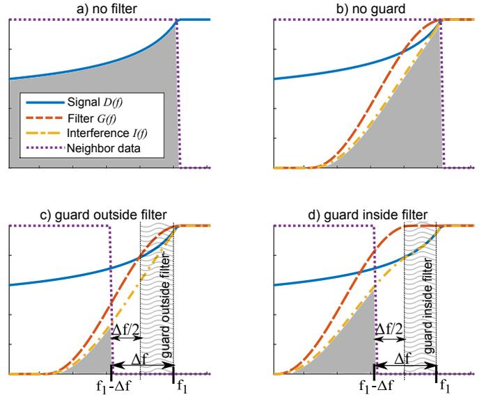
Fig. 5. Guard bands keeping regular resource grid
