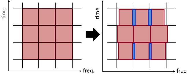
Fig. 3. Guard bands keeping regular resource grid.
