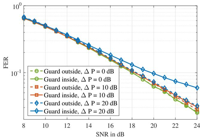
Fig. 11. FER performance for F-OFDM with different number of guard subcarriers, EPA channel, 3 km/h, 16-QAM,  $R_c = 0.55$ , 2 guard SCs.
