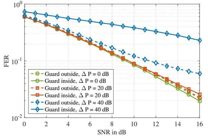
Fig. 10. FER performance for F-OFDM with different number of guard subcarriers, EPA channel, 3 km/h, QPSK,  $R_c = 0.32$ , 2 guard SCs.
