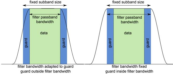
Fig. 4. Two approaches to keep regular resource grid.
