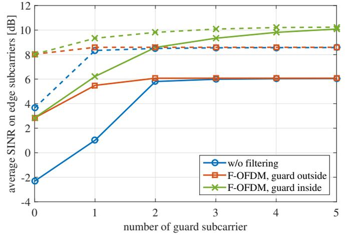
Fig. 7. SINR of edge subcarriers versus number of guard subcarrier for SNR=10 dB, outmost SC (solid) and second outmost SC (dashed)
