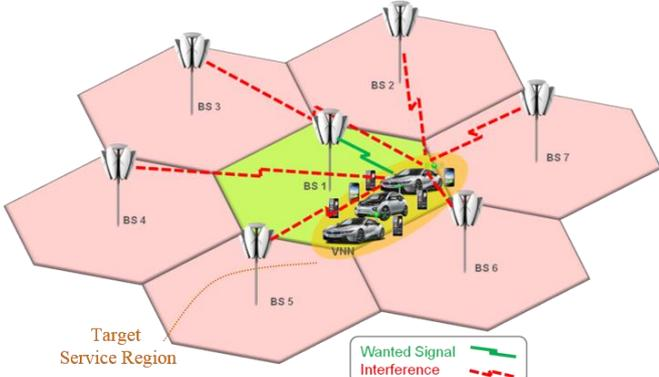
Fig. 1. The considered system model with UEs, VNNs and macro BSs. The active VNN to serve the target service region and the associated serving BS are selected based on the backhaul link SINR.
