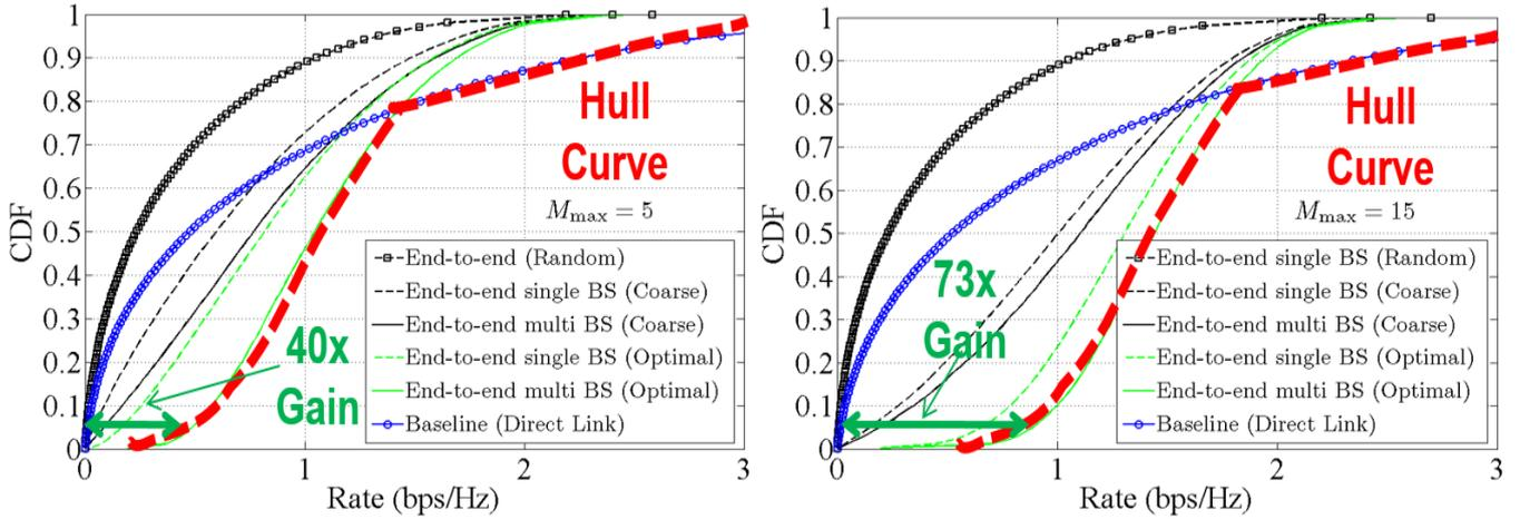
Fig. 3. End-to-end rate gains with different RAN moderation strategies considering  $M_{\max} = 5$  (left) and  $M_{\max} = 15$  (right). The *Hull Curve* indicates the upper bound of achievable gains when the cell selection for the UE (BS or VNN) is optimized.
