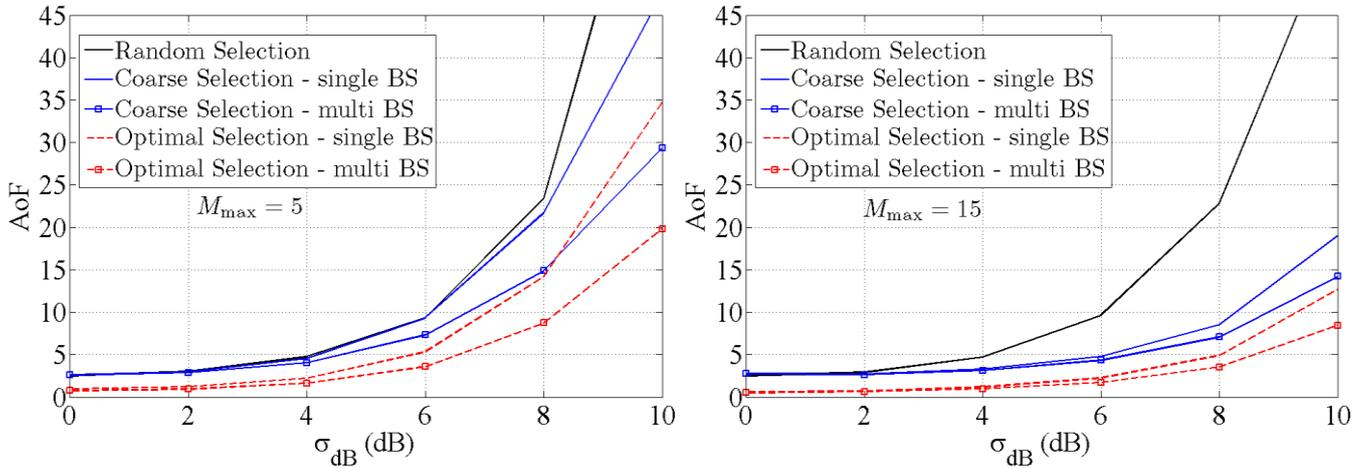
Fig. 4. AoF on the backhaul link as a function of the shadowing standard deviation ( $\sigma_{dB}$ ) on the backhaul link with different RAN moderation strategies considering  $M_{\max} = 5$  (left) and  $M_{\max}=15$  (right).
