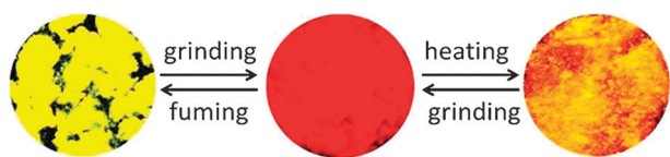
Fig. 2 Switching the solid-state emission of 1 by repeated grinding–fuming and grinding–heating processes. The photographs were taken under 365 nm UV irradiation.
