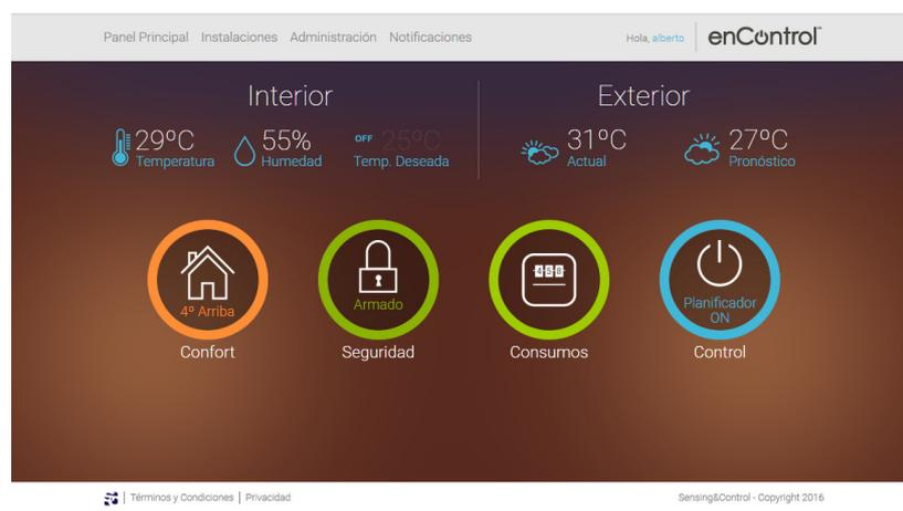
Figure 11: Main screen for all functionalities provided by enControl: comfort, security, energy consumption and automatic control of devices
