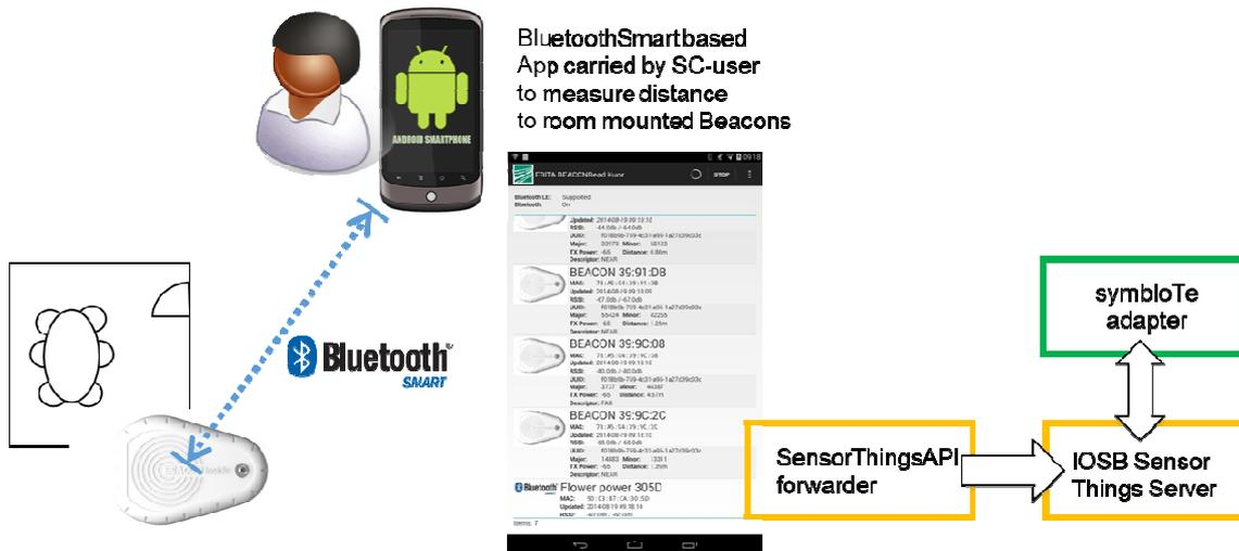
Figure 26: Bluetooth Low Energy based proximity measurement
