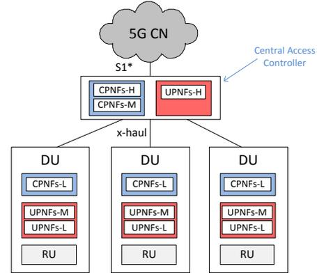
Fig. 4: Deployment with partially centralized control and user plane
