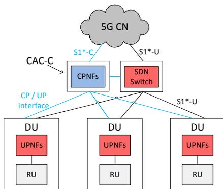
Fig. 3: Deployment with fully centralized control plane
