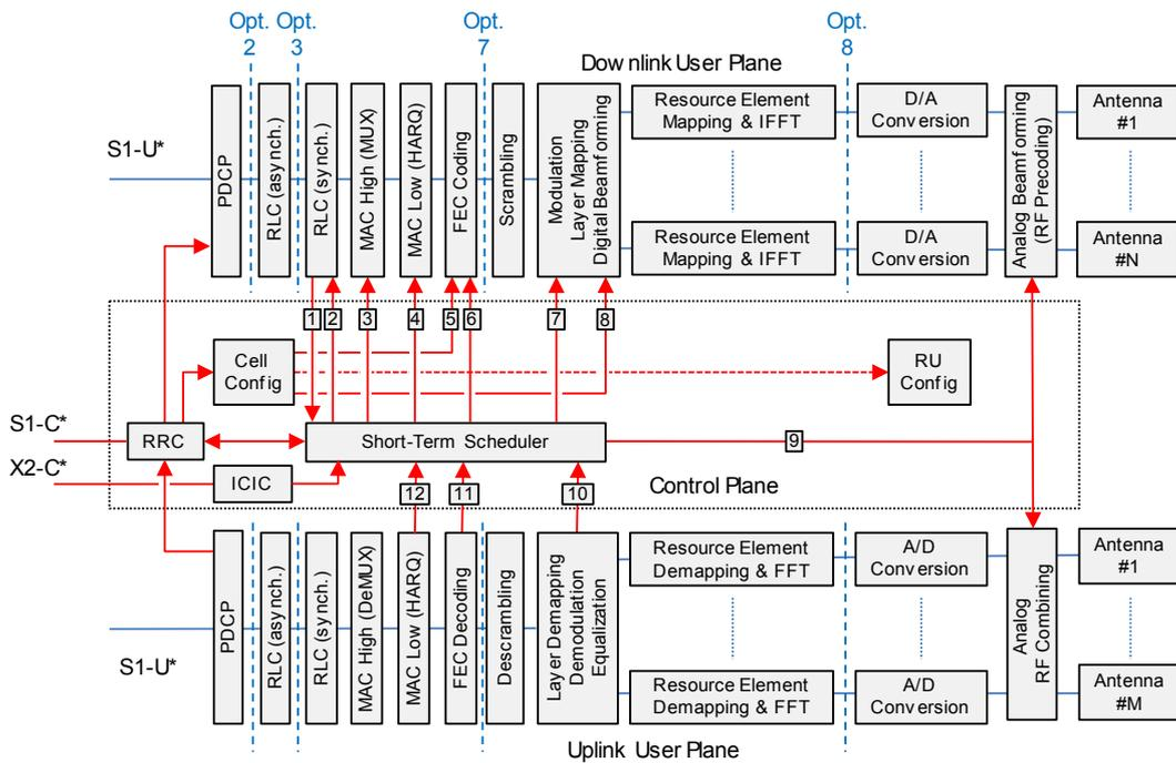
Fig. 2. Control and user plane decomposition and interactions in the radio access network (network infrastructure part only; single radio protocol stack)
