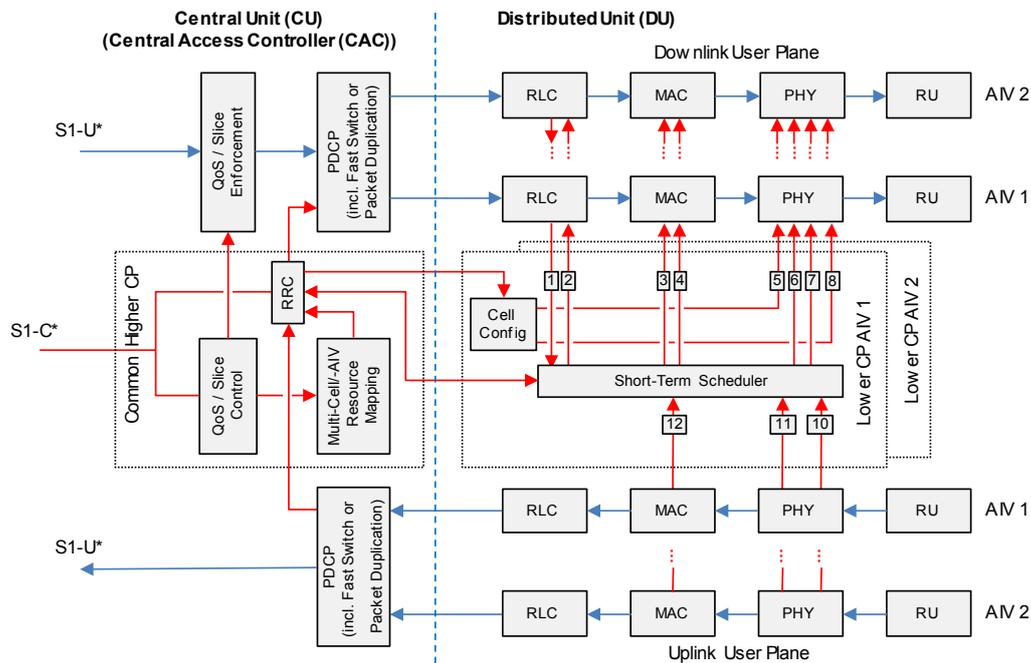
Fig. 5. Partially centralized control and user plane deployment in multi-cell/AIV environment based on horizontal split Option 2
