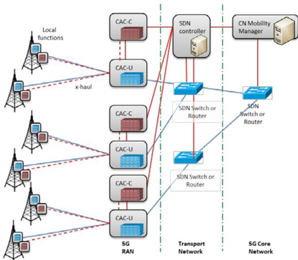
Fig. 1. SDN-based 5G network architecture supporting flexible functional CP/UP splits especially in the radio access (not all CN functions are shown)
