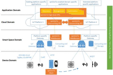
Fig. 1. The symbIoTe high-level architecture.
