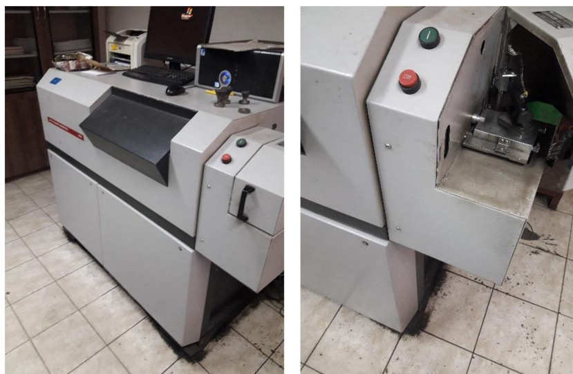
Figure 3. Quantometer Applied Research Laboratories 2460 for chemical analysis.
