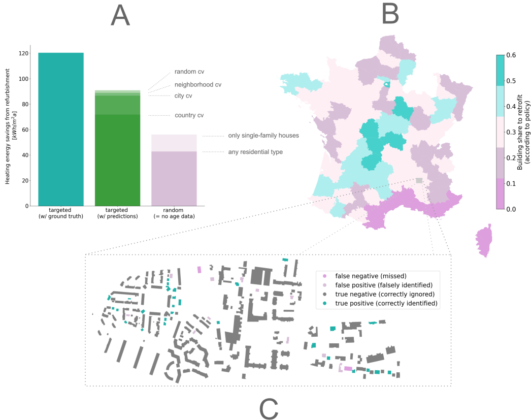
Figure 15: Building age prediction improves retrofit prioritization. Results overview of a targeted prioritization of buildings with a heating demand above 150 \text{ kWh}/\text{m}^2\text{a} . (A) Energy savings per \text{m}^2 of floor space for different levels of knowledge of building age: ground truth knowledge (left), predicted age according to different cross-validation approaches (middle), and no knowledge (right). (B) Regional heterogeneity in the share of buildings in need of retrofitting in France. (C) Illustration of accuracy in determining retrofit needs exemplified by the city of Valence, France.
