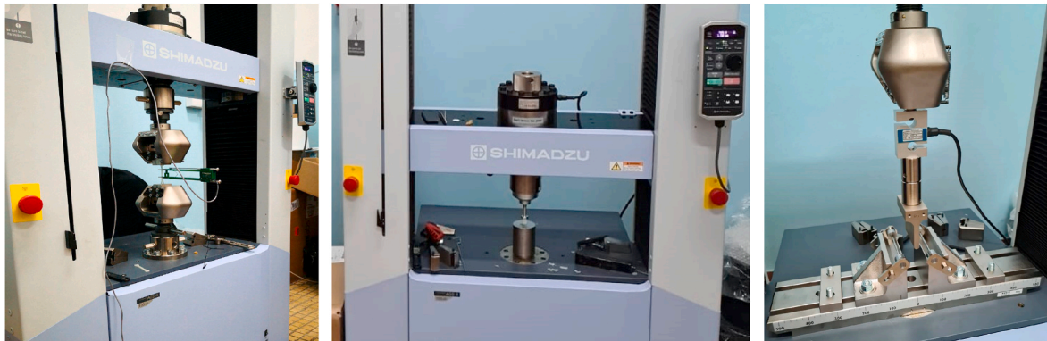
Fig. 5. Shimadzu AGS-X universal testing machine: Left - with loaded tensile testing grips and applied extensometer to tested specimen; Middle - with mounted tools which mimic two plan-parallel surfaces; Right - with mounted adaptors for three-point bending test.
