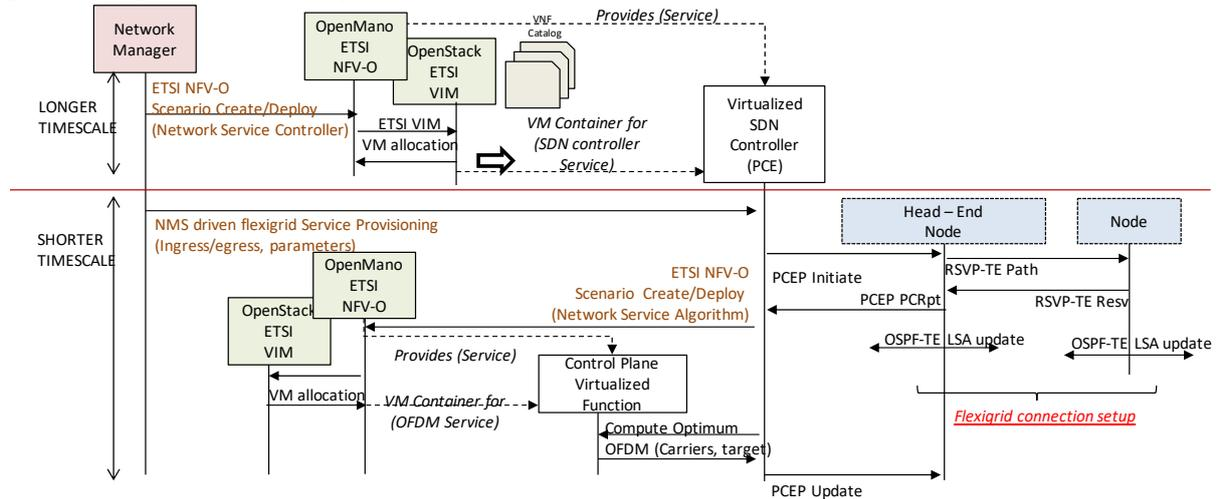
Figure 3. Flow corresponding to the dynamic instantiation of SDN Controllers and CP-specific functions.
