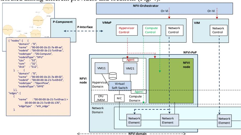
Figure 4. The VIMaP allows delegation of the computation of the VM placement to the P-Component
