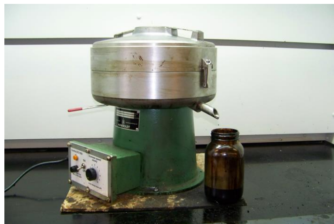
Figure 8-2. Asphalt binder extracted from mixture dissolved in THF
