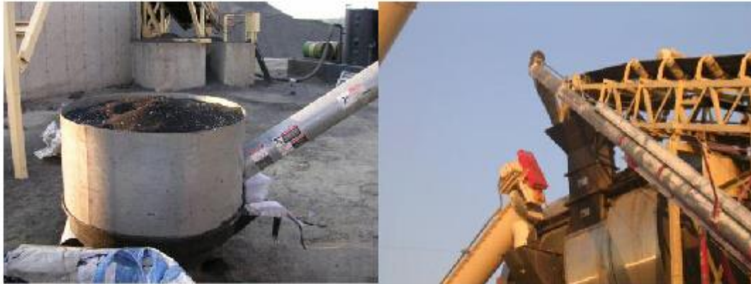
Figure 2-4. Feed system for the dry process ( Hines 2007 )
