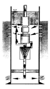
Fig. 4. Downhole oil-water separation schematic [89]
