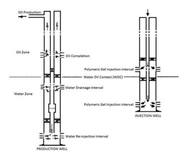
Fig. 8. Well completions of the proposed integrated approach
