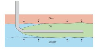
Fig. 3. Horizontal well schematic [82]
