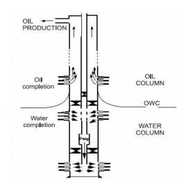
Fig. 6. Downhole water loop schematic [91]
