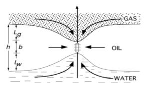
Fig. 2. Gas and water coning schematic in producing well [16]
