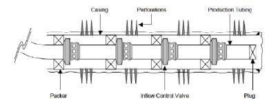
Fig. 7. Intelligent well completion schematic [98]
