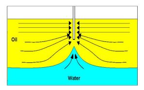
Fig. 1. Schematic of water coning into a well [15]
