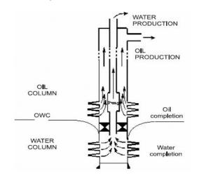
Fig. 5. Downhole water sink schematic [91]
